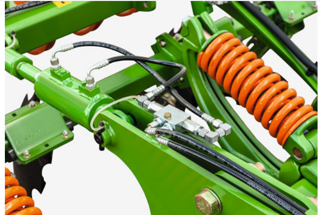
Hydraulic cylinder for setting the depth of the tine section
